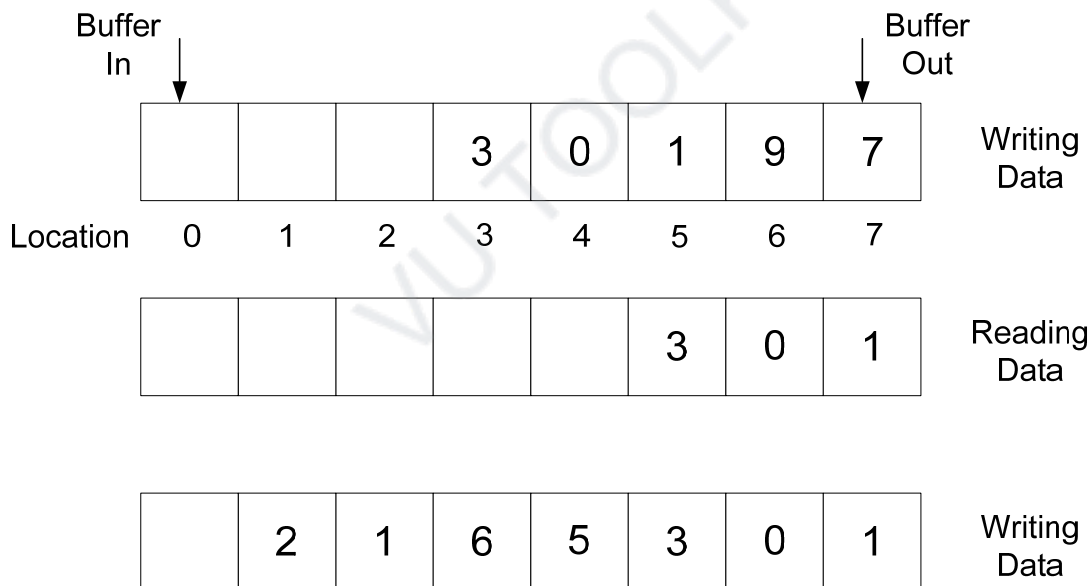
Figure 42.2c Writing and Reading from FIFO Buffer
