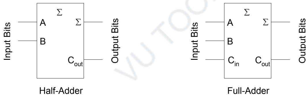
Figure 14.5 Block diagrams of Half-Adder and Full-Adder
