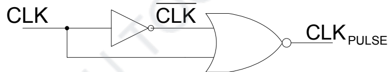
Figure 23.9c Negative clock edge detection circuit
